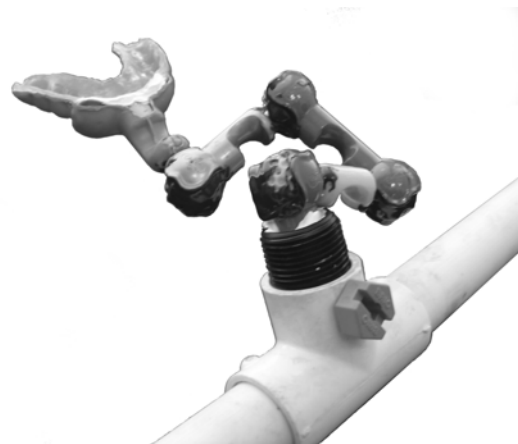
Figure 1. Upper-jaw bite-bar mouthpieces were made for each subject and for each head position. They are attached to a bar that is firmly affixed to the sides of the dewar.
